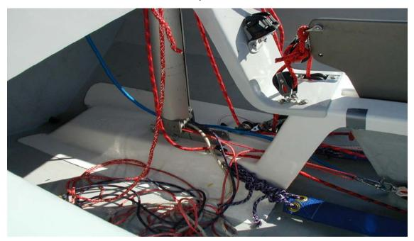
the side tanks and cleats. The centerboard purchase system is 3:1 and most of its components can be seen in this photo. Some sailors have gone to a 2:1 system with the lighter aluminum board. If you are rigging a steel board I recommend at least 4:1 with 6:1 being optimal. Please excuse the messy lines as I took these photos while de rigging the boat after the 2004 Crystal Bowl Regatta.
