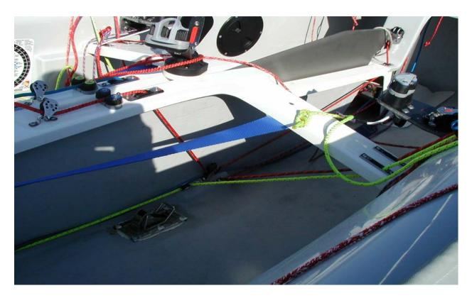
This picture shows the main halyard cleat mounted to the inside of the trunk upright. Also shown is the jib cloth tensioner.
